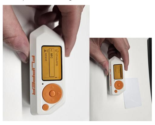
The task was to read and emulate a access card using Flipper Zeros NFC module.
