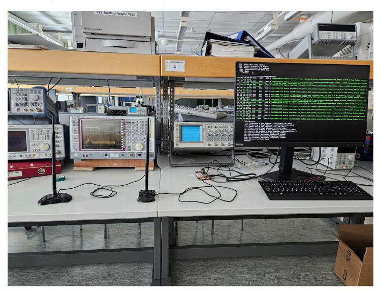
The test-setup above was quite simple. One spectrum analyzer and the CaribouLite-RaspberryPi combo with antennas.
